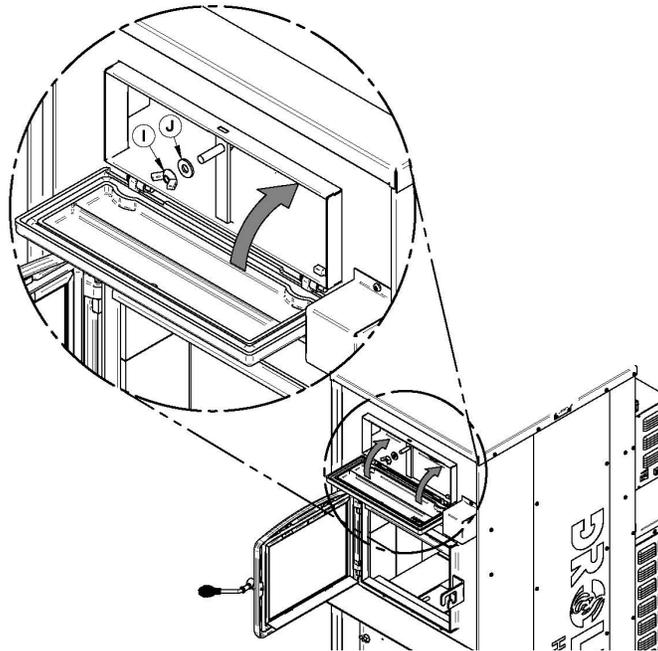
8. If you have performed maintenance from the back part of the furnace, reinstall the black pipe connector and secure it with three screws.
