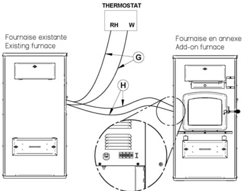
**Step 2.** From the thermostat connected to the existing furnace, connect 2 new wire (**H**) on the Rh and W terminals of your thermostat and fix them to the terminal on the circuit board labeled "I" (interlock) of the Add-On furnace.
