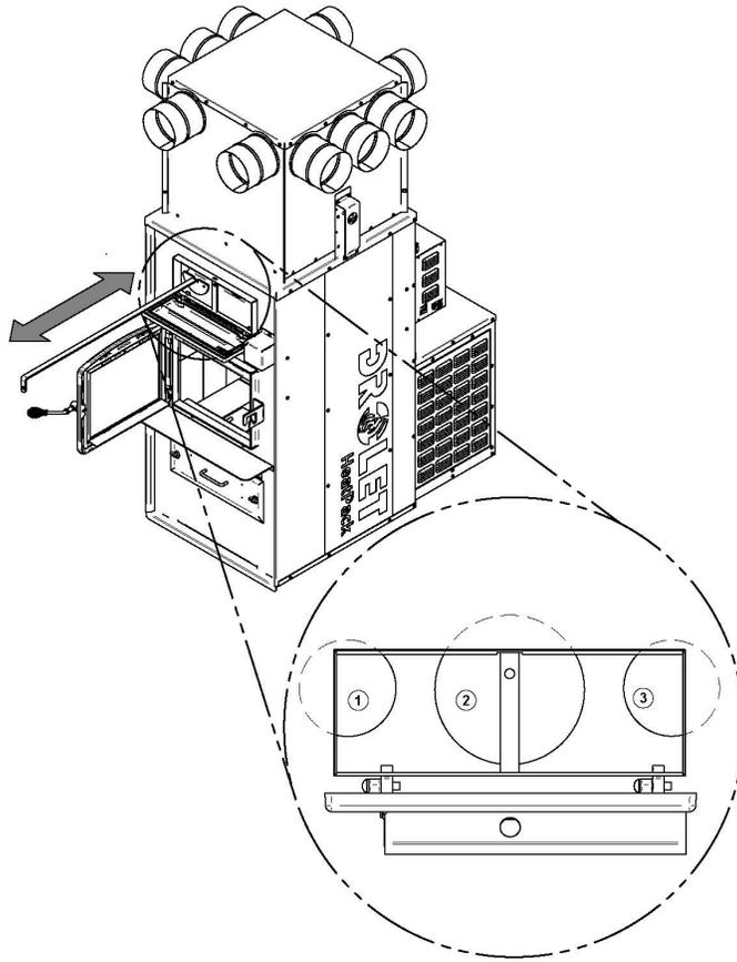
4. Dirt in the exchangers 1 and 3 fall into the combustion chamber, at the rear.
