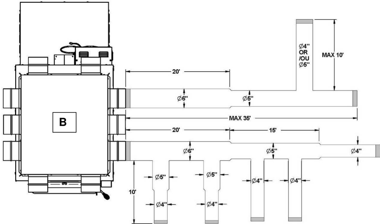
The total area of secondary duct outlets must be equal or slightly less than the total area of the outlets used on the hot air distribution plenum (**B**).
