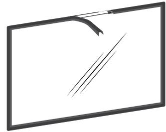
9. Install the glass (E) and glass frame (D) centering them in the door frame. Install the glass retainers (C) taking care not to over tighten the screws (B). Note that the two main causes of glass breakage are unequal position in the door and screws too tight.
