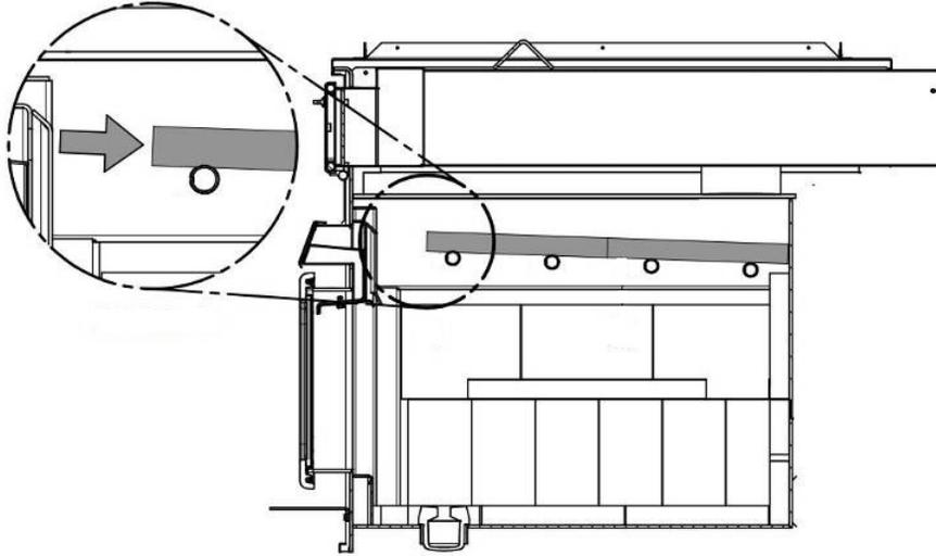
7. Close the exchanger access door and secure it using the washer (C) and wing nut (B).
