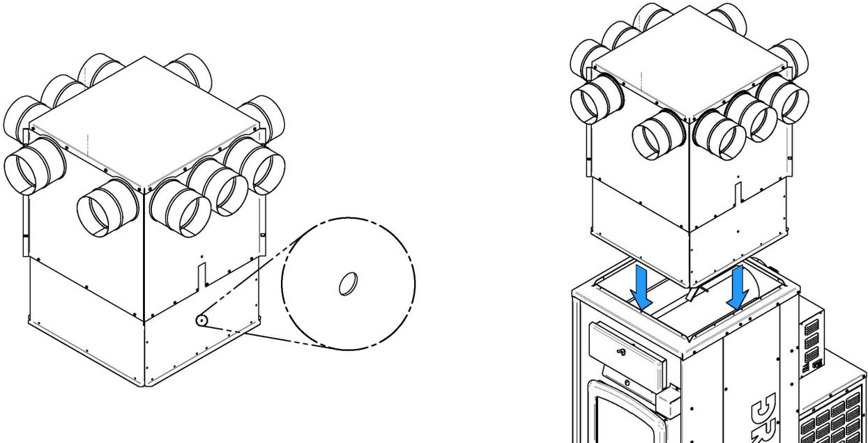
**Step 3 :** Using 14 black screws (C) #10 x 5/8", secure the plenum to the furnace.
