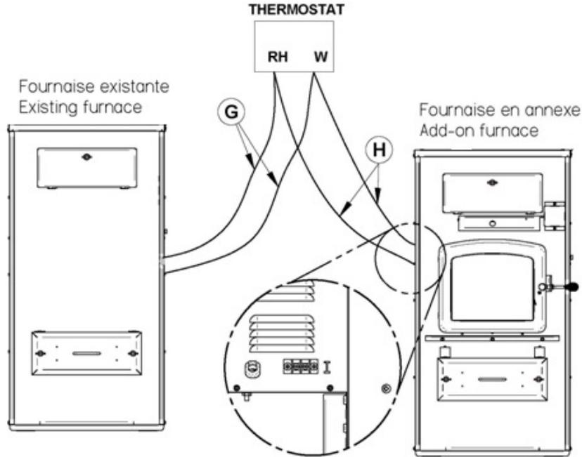
When the wood furnace receives the signal from the existing furnace's thermostat calling for heat, it will disconnect the existing furnace damper motor, sending the wood furnace in low burn until the call for heat from that thermostat is satisfied.
