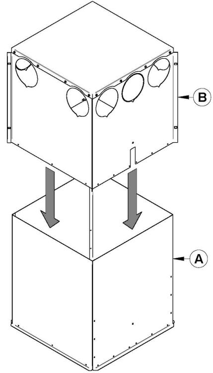
Using 13 self-drilling screws, secure the plenum (B) to the plenum extension (A).
