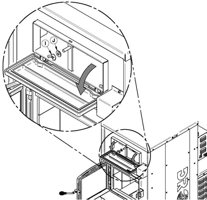
2. Move the baffle **(K)** of the combustion chamber forward.
