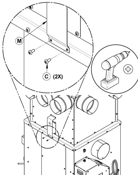
**Step 3.** Pre drill the two top RTD probe support holes with a 1/8" drill bit in the furnace plenum. Secure it in place with two screws (C).
