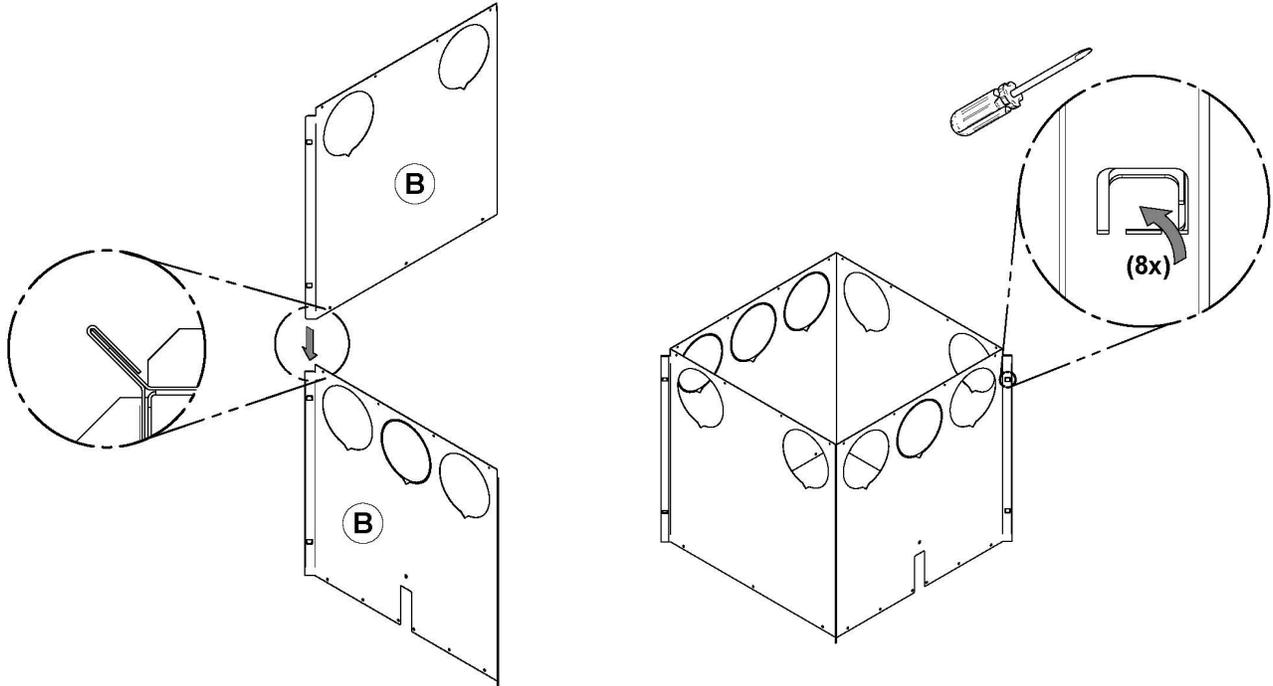
**Step 3:** Install the cover (B) and secure it with 16 black screws (C) #10 x 5/8" robertson type A, provided in the user manual.
