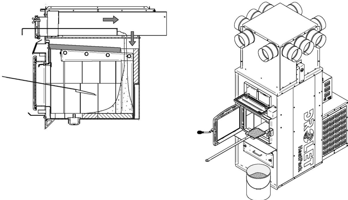
5. Dirt in the central exchanger (2) will be removed from the front or the rear of the furnace. If you remove dirt from the central exchange to the back of the furnace, remove the black pipe connector in order to dispose of the dirt.
