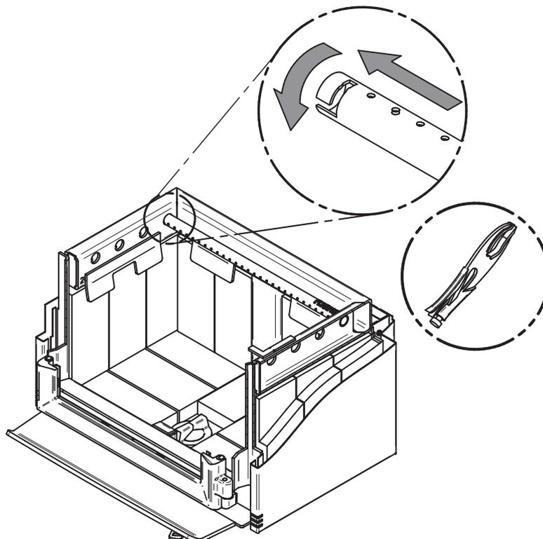
Note that secondary air tubes (B) can be replaced without removing the baffle board (A) and that all tube are not necessarily identical (look at the part number on the tube).
