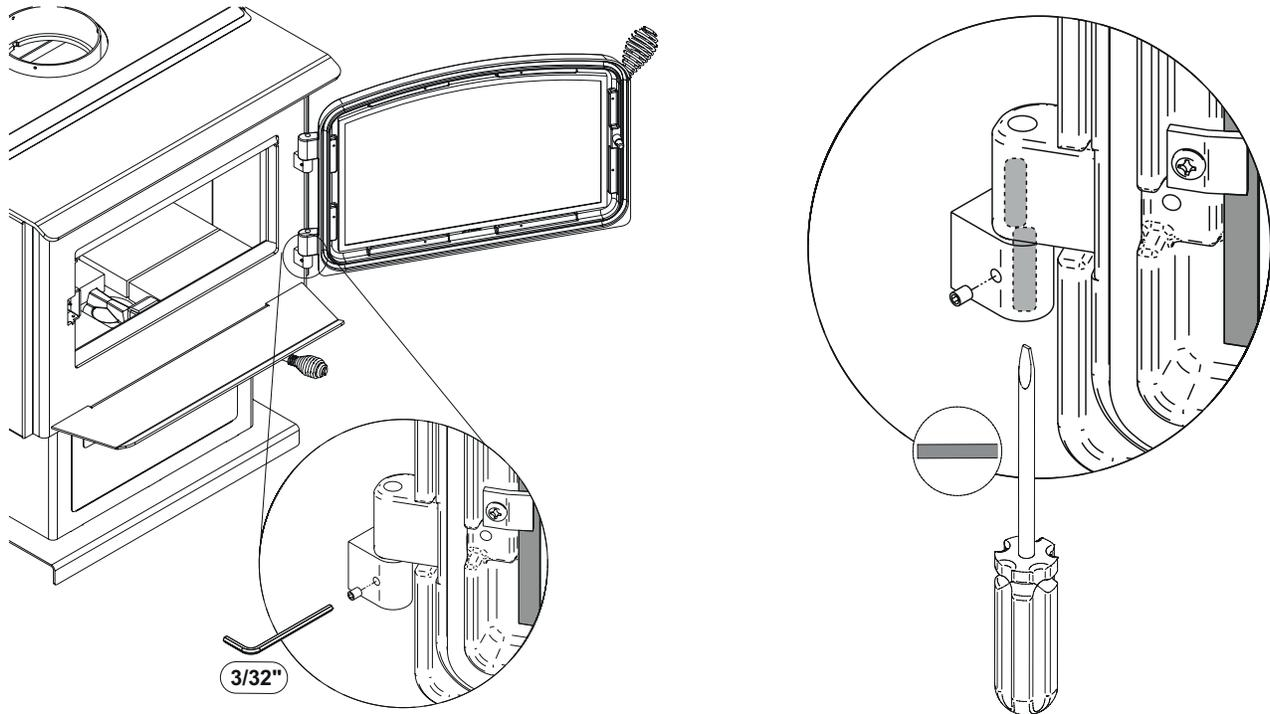
Using a flat screwdriver, turn the adjustable hinge rods in the direction shown to adjust the doors. Tighten all door hinge pressure screws when they are at the desired positions. Configurations 1-2-3-4-5-6, show in which direction these act on the adjustment of the door.
