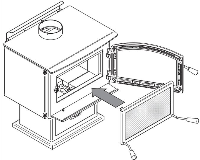
3. Lean the upper part of the fire screen against the top door opening making sure to position the top fire screen brackets behind the primary air deflector.
