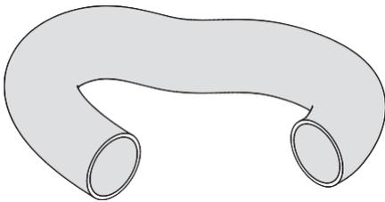
Tuyau isolé flexible de type HVAC
