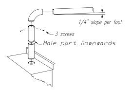
Your smoke evacuation system (pipes) should be assembled in such a way that the male section of the pipes faces down. Attach each of the sections to one another with three equidistant metal screws. The pipes must be short and straight. All sections installed horizontally must slope at least 1/4 inch per foot, with the lower section toward the stove.
