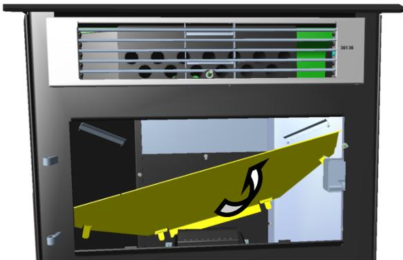
3. Rotate the baffle and align the right corner to the upper right corner of the door opening.
