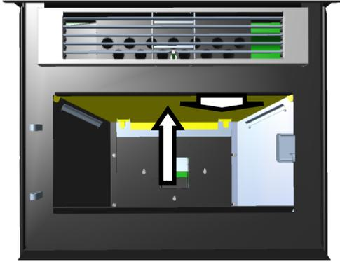
1. Lift the baffle and slide forward it a little to clear the supports.
