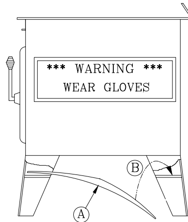
4. A- BEND SLIGHTLY HEAT PROTECTOR AND B- PUSH IT BACK IN PLACE ON THE SUPPORTS
