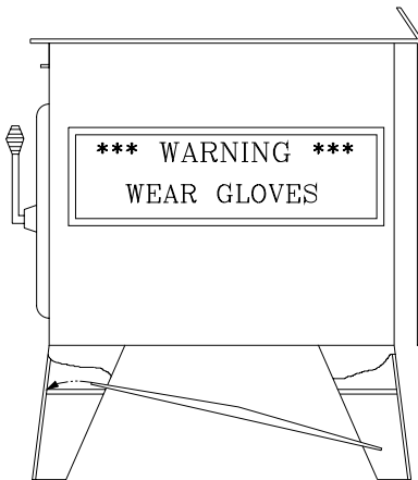
3. SEAT HEAT PROTECTOR BETWEEN FRONT LEGS ON THE SUPPORTS
